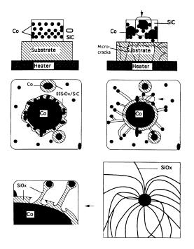
**Fig. 9** Nanoflower growth model: (a) Heating assembly; (b) Fissured  $SiO_2$  and agglomerated Co; (c) Spherical Co particles; (d) Initial growth stage; (e) Magnified nanotube growth; (f) Final stages of growth.
