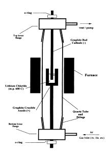
Fig. 4 Electrolysis set-up.
