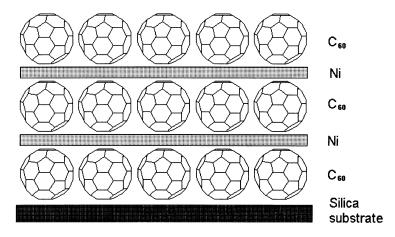
Fig. 10 Thin layers of successively deposited pure Ni and  $C_{\rm 60}.$
