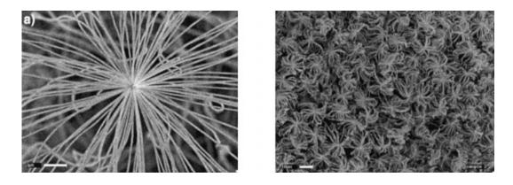
**Fig. 8** (a) SEM image of a single silica nanoflower exhibiting radially attached fibres to a central sphere. (b) SEM image of a silica nanoflower film produced in the presence of CO.
