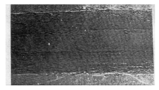
**Fig. 6** High resolution transmission electron micrograph showing the degree of graphitisation of an electrolytically formed multi-walled carbon nanotube. The interlaying spacing of the graphene sheets is 0.34 nm.
