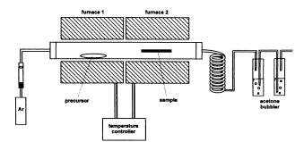
Fig. 2 Pyrolysis set-up.
