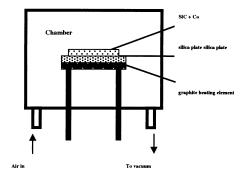
Fig. 7 Furnace assembly.
