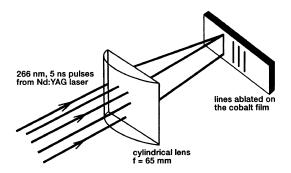
Fig. 1 Laser etching set-up.
