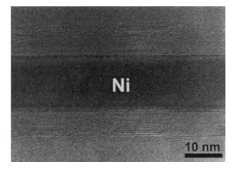
Fig. 12 HRTEM image of a highly graphitised Ni-filled carbon nanotube. The quality of graphitisation is unusual for pyrolytically grown materials.
