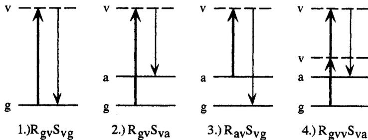
Fig. 6. Examples of Rayleigh and Raman scattering
