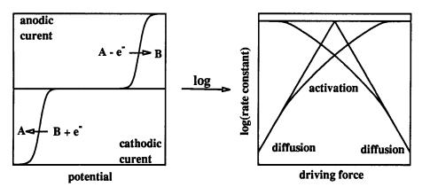
The continuous lines drawn in the figure are an almost exact representation of reality since the driving force can be changed, through the electrode potential, almost continuously with a precision of the order of
