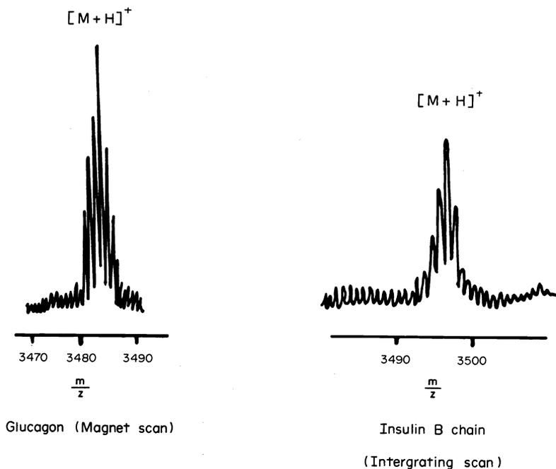
Fig. 11. Molecular ion regions of the FAB spectra of Glucagon and the Insulin B chain. Quasimolecular ions obtained in each case.
