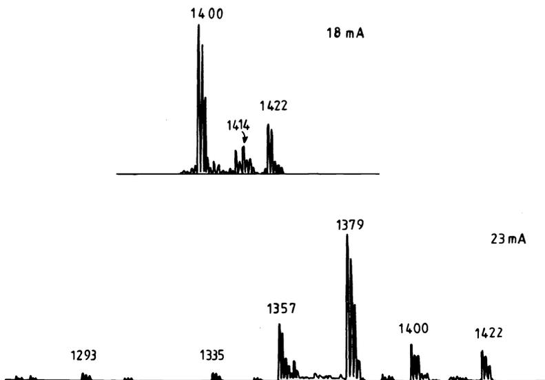
Fig. 5. The FD spectrum of Bleomycin demethyl A<sub>2</sub>. The emitter current was increased from 0-30mA. An intense quasimolecular ion ( $M+H^+$ ,  $m/z$  1400) was observed at 18mA with fragmentation occurring at 23mA.
