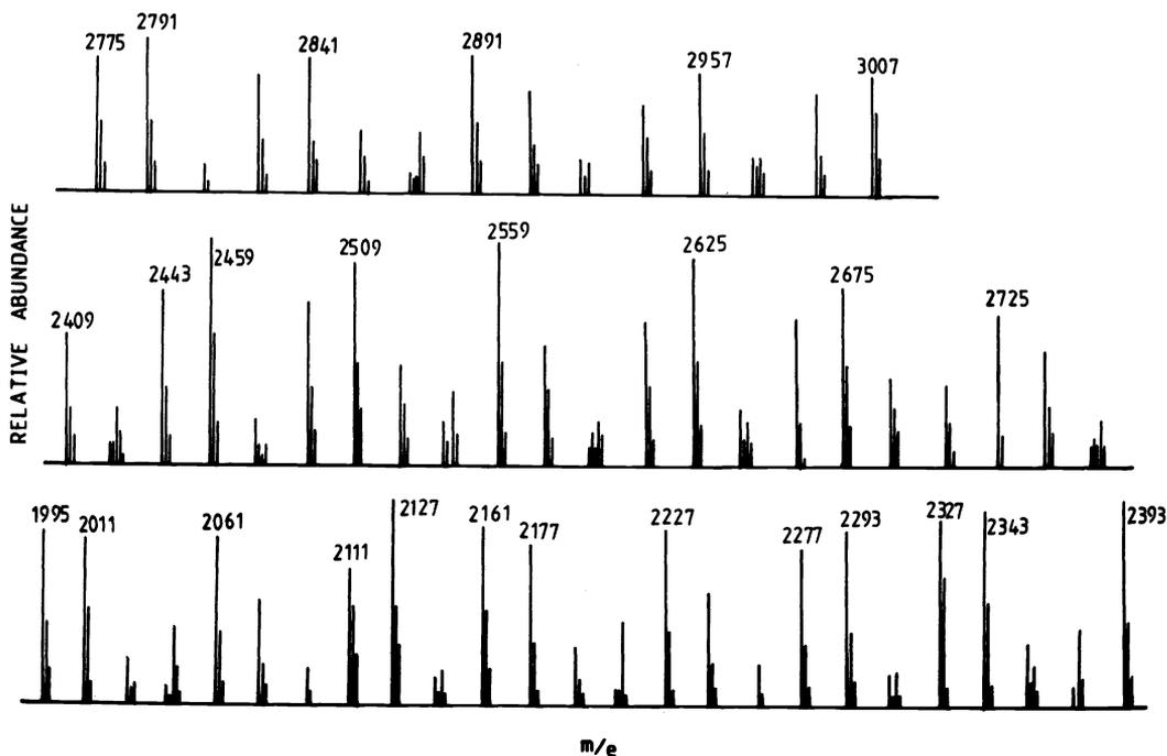
Fig. 4. NCI spectrum between  $m/z$  2000-3000 of Fomblin oil. This material is also used as a high mass reference for FD MS studies.
