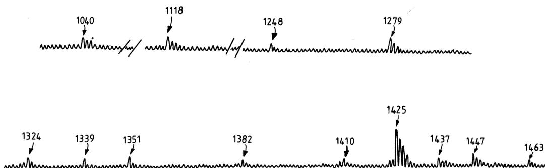
Fig. 6a. Fast Atom Bombardment spectrum of Bleomycin B<sub>2</sub> showing the quasimolecular ion (M+H<sup>+</sup>, m/z 1425) and fragment ions above m/z 1000.
