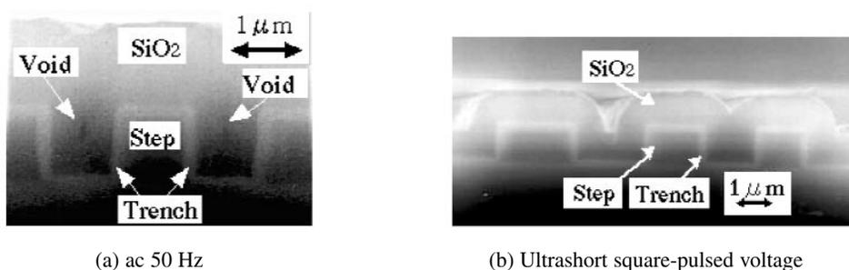
**Fig. 3** SEM micrographs of SiO<sub>2</sub> film deposited on trenches having an aspect ratio of 0.8.
