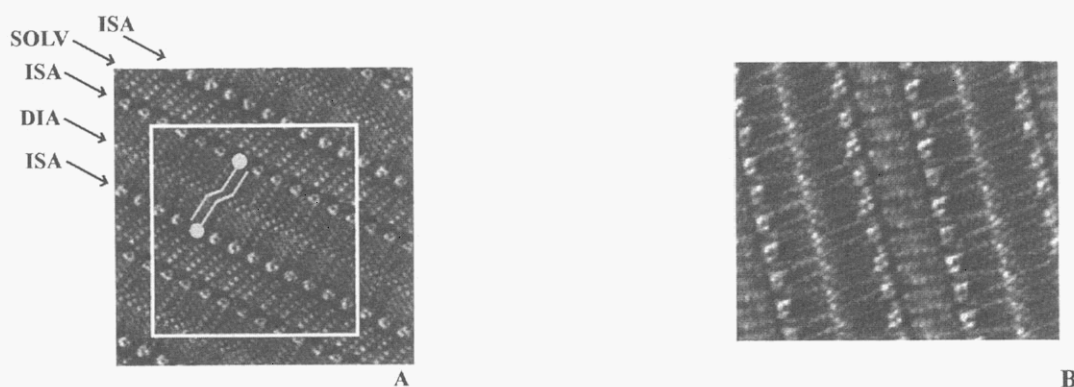
Figure 13. A. An STM image of a physisorbed monolayer of ISAC 9 (DIA)C 10 molecules from a solution in 1-undecanol, image size 12.7 x 12.7 nm 2 . White corresponds to the highest and black to the lowest measured tunneling current in the image. Bias voltage and average tunneling current were -1.2 V and 1.0 nA, respectively. B. An STM image of a polymerized monolayer structure. White corresponds to the highest and black to the lowest measured tunneling current in the image. Image size: 10.8 x 10.8 nm 2 . Bias voltage and average tunneling current were -0.5 V and 1.0 nA, respectively.
