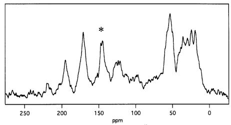
Fig. 3 CP/MAS spectrum of  $\alpha$ -crustacyanin reconstituted with [12,12'-<sup>13</sup>C<sub>2</sub>] astaxanthin, recorded at  $\omega_r/2\pi = 6.00$  kHz, at a sample temperature T  $\sim$  230 K.
