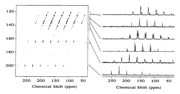
Fig. 2 TOSS - reversed TOSS spectrum of all-E-astaxanthin, collected with  $\omega_r/2\pi$  =2750 Hz. To the right are shown projections of regions of the 2-D dataset.
