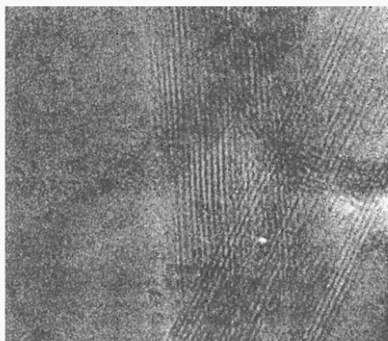
Fig. 1 Single-walled nanotube ropes. Fringes are spaced by about 1.2 nm in both figures.
