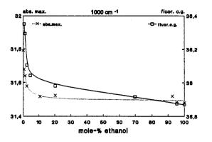
Figure 2: Absorption maximum and the center of garvity of the fluorescence spectrum of catechol in n-hexane binary mixtures with ethanol.
