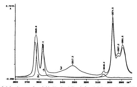
Figure 3: Infrared spectra of catechol in (1), ethanol (2) and of catechol plus ethanol (3) in CCl<sub>4</sub> solution.
