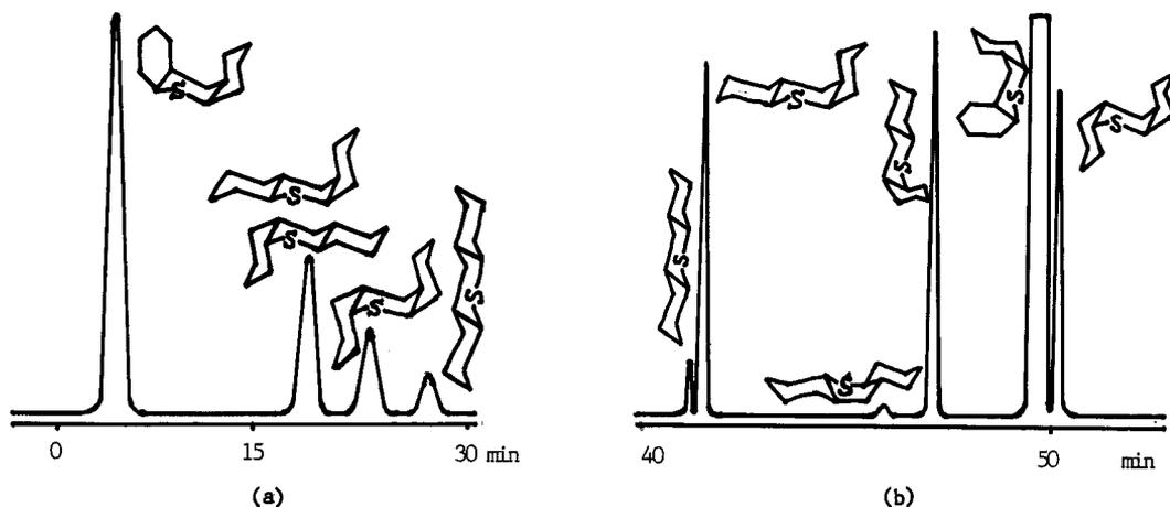
Fig. 1. Chromatogram of PHTX: (a) GTCB, 2m x 1mm, temperature programming 200° to 280°C, 10/min; (b) SP-1000, 50 m x 0.25 mm, temperature 145°C.
