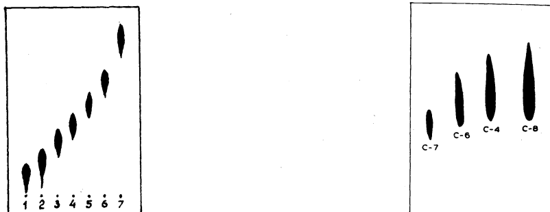
Fig.1. TLC of random copolymers of styrene (St) and acrylonitrile (AN) containing (1) 41%, (2) 34.1%, (3) 27.6%, (4) 19.3%, (5) 14.7%, (6) 8.7% and (7) 0 AN. A system with gradient from a mixture of tetrachloromethane and acetonitrile (6.5:0.5) to acetonitrile.
