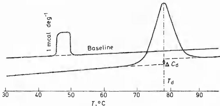
Figure 4. Microcalorimetric recording of heated lysozyme solution. The concentration of the solution was  $1.6 \text{ g l}^{-1}$  (ref. 19).
