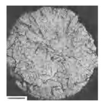
Figure 13. Electron micrograph of the fracture surface of pressure crystallized polyethylene as in Figures 11 and 12 showing the spherulitic development. Scale 10 µm. (Ref. 15)
