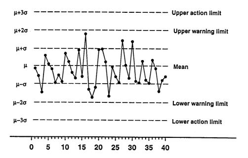
Fig.18.6.1 Results from a system in statistical control
